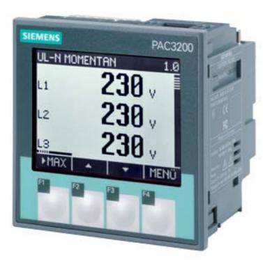
SENTRON PAC3200; LCD; 96X96MM POWER MONITORING DEVICE PANEL MOUNT TYPE FOR MEASUREMENT OF ELECTR. VALUES VAUX: 110-340VDC / 95-240VAC VIN: MAX.690/400V; 45-65HZ AMPIN: X/1A OR X/5A AC COMPRESSION TYPE TERMINALS
