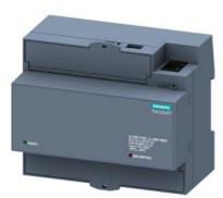
SENTRON, measuring device, 7KM PAC3200T, strd mnt. rail encl. w/o display, L-L: 400 V, L-N: 230 V, 5 A, strd rail instr., 3-phase, MODBUS TCP, apparent /active/reactive energy, wide-range pwr sup. unit AC/DC, screw terminals
