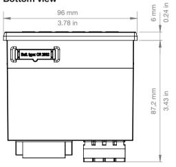
Cut-out dimension: 92<sup>+0.8</sup> mm x 92<sup>+0.8</sup> mm (3.62<sup>+0.03</sup> in x 3.62<sup>+0.03</sup> in)
